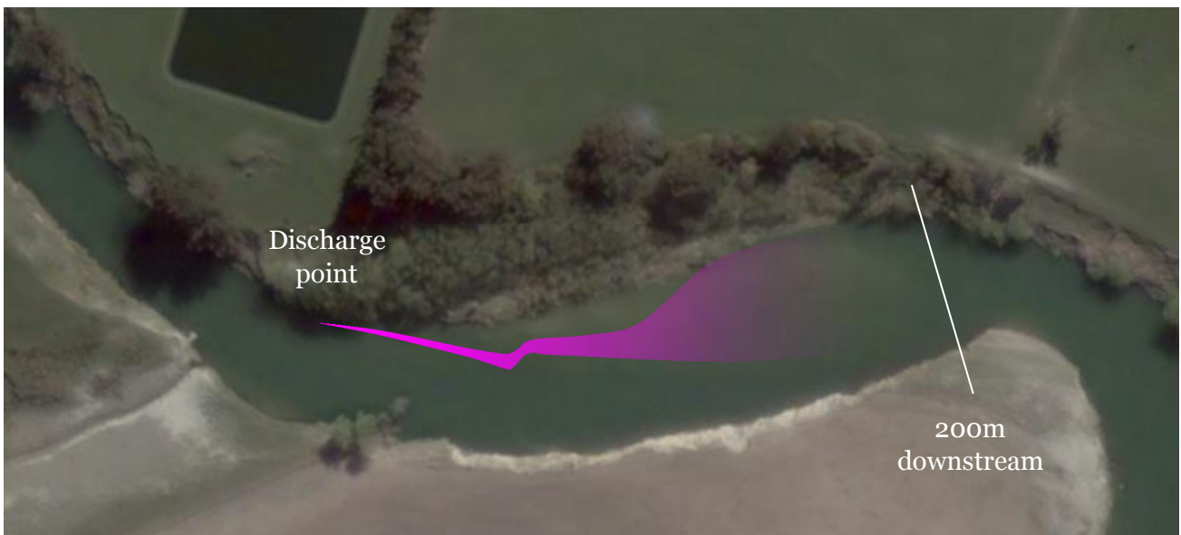
Figure 1.2: Sketch of Porangahau township WWTP effluent discharge plume in Porangahau River on outgoing tide based on a visible dye trace. The white line indicates the distance 200m downstream of the discharge point.
