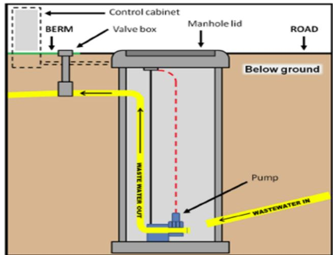
Wairoa’s wastewater reticulation includes five pump stations that service different catchment areas of the wastewater reticulation network. Under extreme weather conditions (discussed below) the flow into some pump stations exceeds the ability for it to be discharged and pump station overflow occurs.
