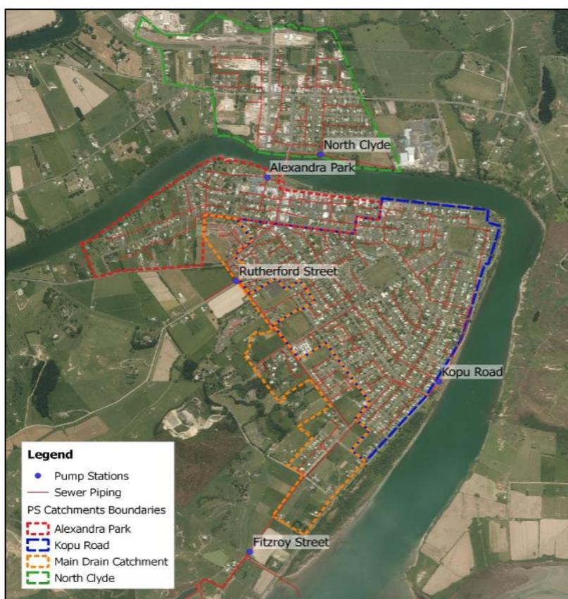
Reticulation is designed like an underground version of a stream with a single large pipe at the final downstream end that is fed by incoming branches of large pipes (**mains**) that split upstream into more and more branches and sub-branches with smaller and smaller pipe diameters to match the smaller flow rates. Each area of reticulation that ultimately flows into a common main is called a **catchment**.
