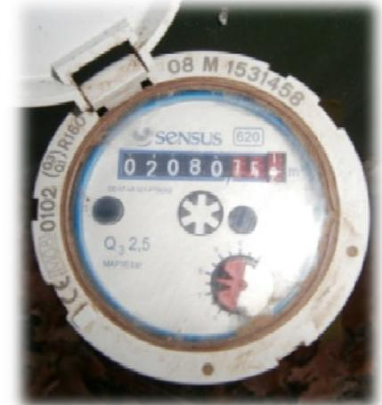
The above meter has a reading of 2080.75. The black dials with white numbers are cubic meters and the red dials with white being Litres, working right to left
