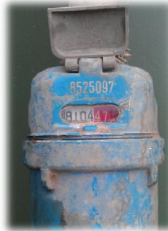
The above meter has a reading of 8104.477. The white dials with black numbers are cubic meters and the red dials with white numbers (units) being litres. Working right to left
