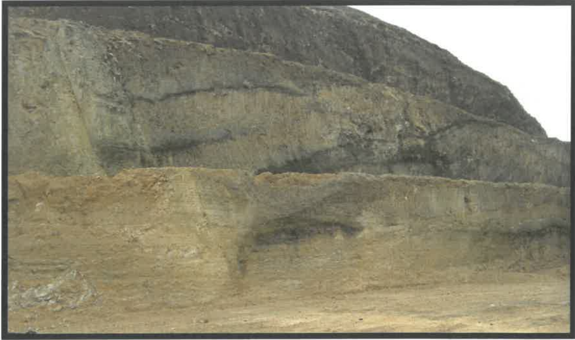
View of Hatuma Lime's Mauriceville quarry showing quarry bench (x 3) and faces
