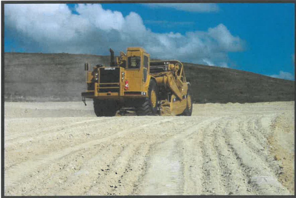
Catepillar 639D Elevating Motor-Scraper harvesting raw limestone
