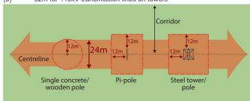
The National Grid Subdivision Corridor and National Grid Yard do not apply to underground cables or any underground transmission lines (or sections of line) that are designated by Transpower. The measurement of setback distances from National Grid lines is to be taken from the centre line of the two support structures at each end of the span.
