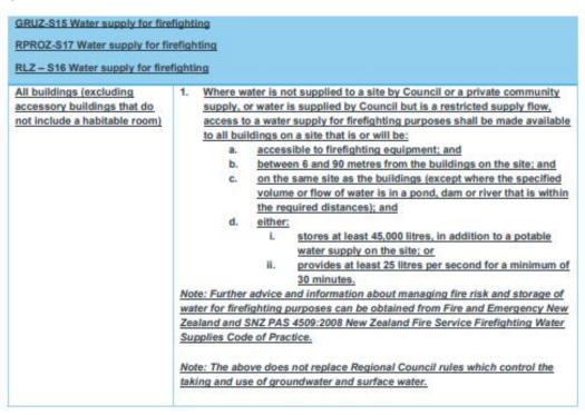
This proposed provision sets out the minimum requirements for Fire Water Classification 2 (FW2) of the New Zealand Fire Service Firefighting Water Supplies Code of Practice SNA PAS 4509:2008 (Code of Practice) and would apply to permitted activities listed in the GRUZ-General Rural Zone, RPROZ – Rural Production Zone and RLZ – Rural Lifestyle Zone chapters. As per the Code of Practice, FW2 is considered sufficient firefighting water supply for:
