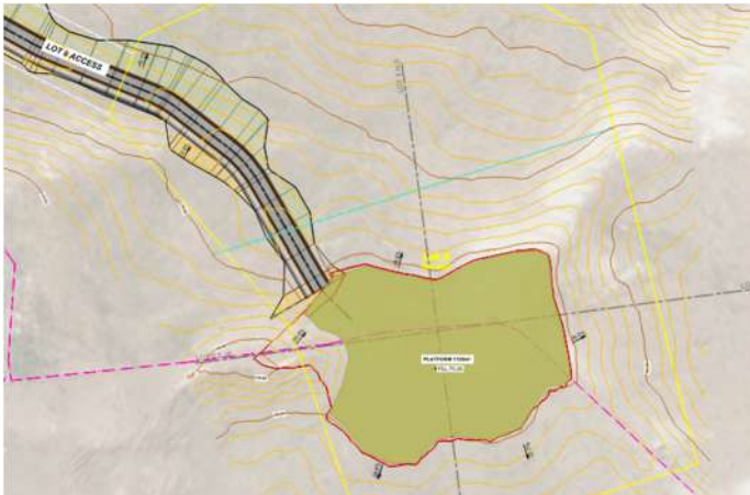
Figure 21 - Lot 8 platform and Catchment flow direction
