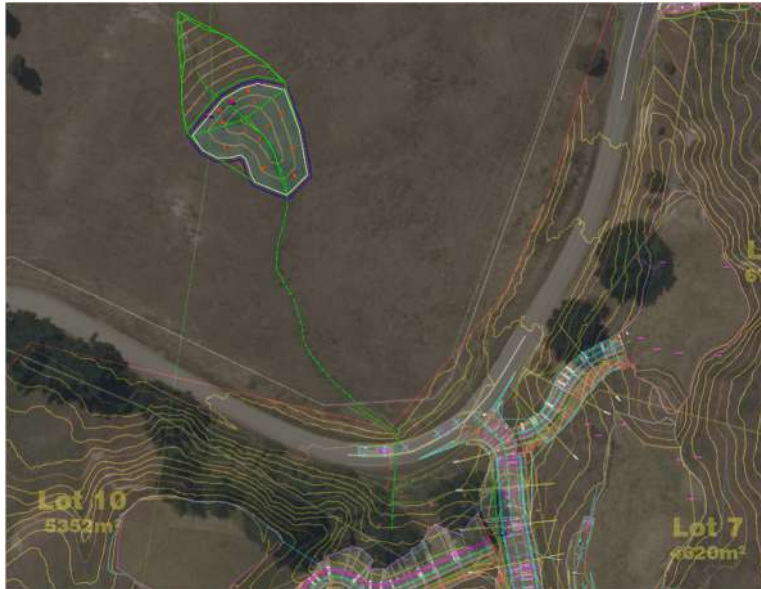
Figure 24 - Dry stormwater pond B - north of Williams Road
