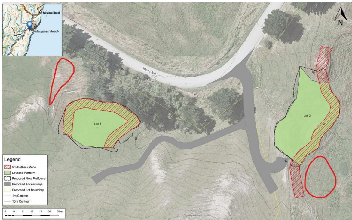
Figure 8: Excerpt from RDCL Geotechnical Report showing vehicle access, building platforms (green zones), 5m setback zone (red shaded) with approximate effluent disposal field locations overlaid (red circles).
