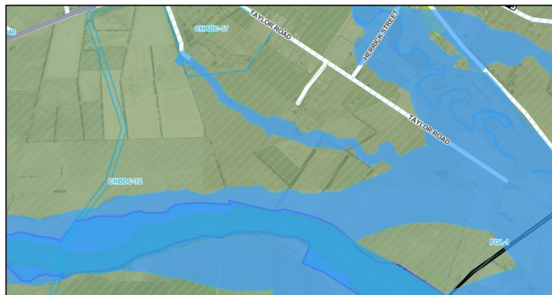
Figure 19: Image showing the flood hazards on the site.
