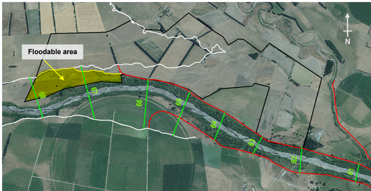
Figure 4: Cross-sections (green lines) from HBRC 1D model.
